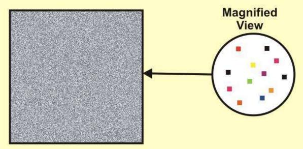
This is visible in an x-ray image as noise (quantum noise).
