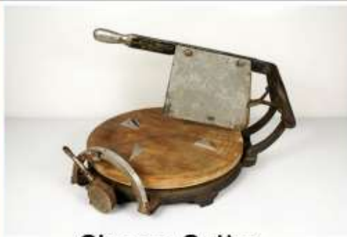
Cheese Cutter Gauge measures size to be cut.
